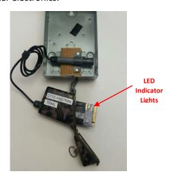
4. When operating normally, the RED LED indicator light (see below) should flash once every 5 seconds. The GREEN light should flash when, and only when an object passes the counter. Wave your hand in front of the sensor to make sure it is working. Do not touch the exposed metal contacts:
